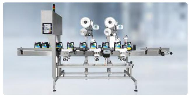
Arca is an Italian manufacturer of industrial automatic labeling systems and laser marking systems with 20 m/min to 150 m/min speed.
